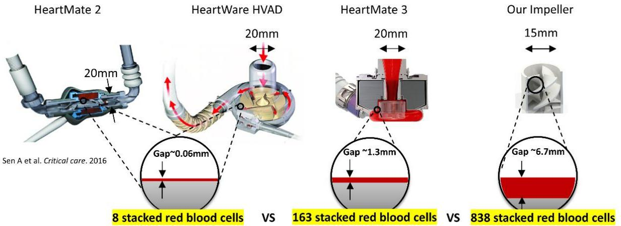
**Fig S5. Blood flow gap size comparison.** The number of blood cells that can be stacked inside the BiO-H is 838 compared to 8 and 163 for the HeartMate 2 (Abbott, Chicago, IL) or HeartWare HVAD (Medtronic, Minneapolis, MN) and HeartMate 3 (Abbott, Chicago, IL).
