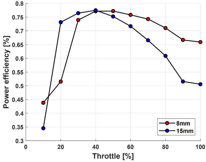
**Fig S4. Power efficiency measurements.** Voltage and current were measured at motor terminals for each throttle to calculate power efficiency by following Eq 2. The small and large pump prototypes show different power efficiency profiles although the same motor has been used due to the load differences between the two.
