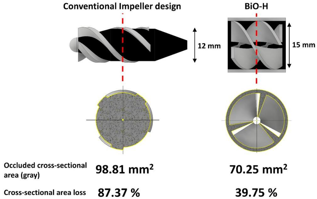
**Fig S6. Occluded cross-sectional area comparison.** BiO-H shows 2.25-fold less cross-sectional area loss than the conventional impeller design (e.g. HeartMate II)
