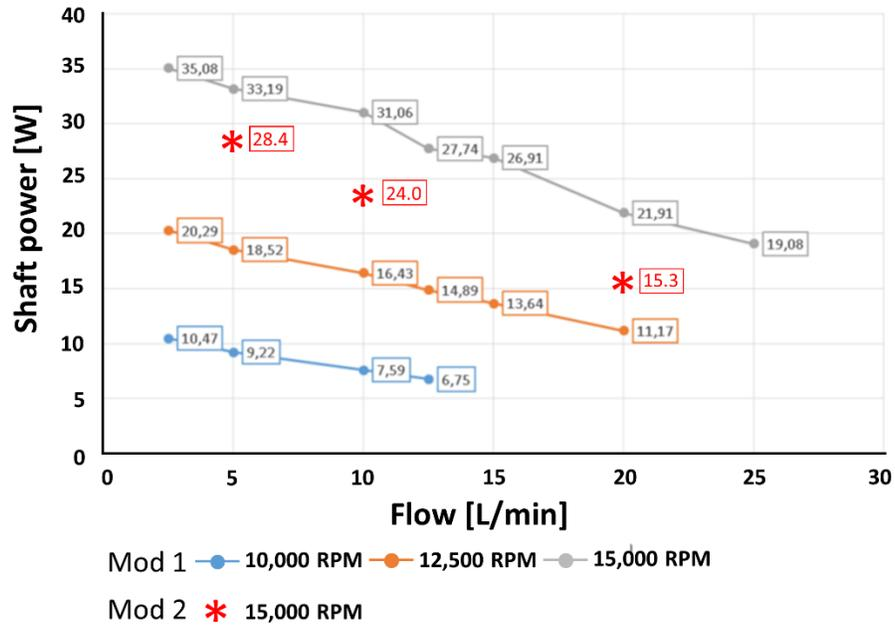
**Fig S2. Shaft power resulted from Mod 1 and Mod 2.** Shaft power is an integral of hydraulic power plotted in Fig 7 as a variable over the blade surfaces which visualizes the efficiency of the flow guidance and highlights areas where hydraulic losses occur.
