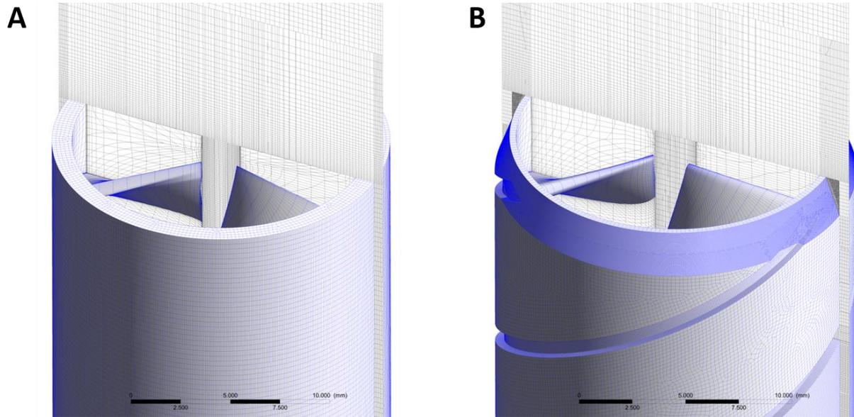
**Fig S1. Mesh images for Mod 1 and Mod 2.** The mesh consists of 4,418,397 elements and 13,299,271 elements for Mod 1 and Mod 2 respectively. The meshing of Mod 2 required more mesh regions to ensure a sufficient mesh quality in the gap, the additional chamfers, the troughs on the outside, and the roundings at the leading edge; these additional features resulted in larger elements.
