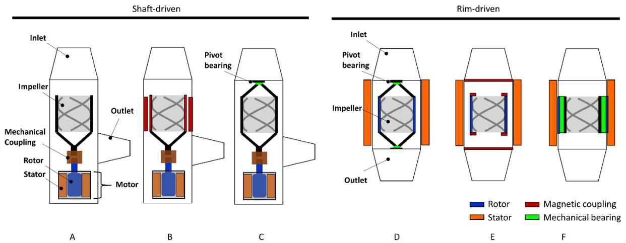
**Fig S7. Actuation mechanism.** (A) Shaft-driven mechanism with mechanical coupling. (B) Shaft-driven mechanism combined with magnetic coupling. (C) Shaft-driven mechanism combined with pivot bearing. (D) Rim-driven mechanism with pivot bearings. (E) Rim-driven mechanism with a fully magnetically levitated system. (F) Rim-driven mechanism with a structurally integrated mechanical bearing between impeller and housing.
