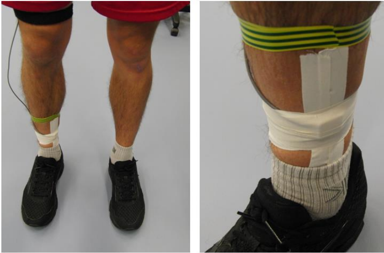
Figure SDC 1. Example of the attachment of the accelerometer taped to the tibia of the right leg of the participant during the experiment.
